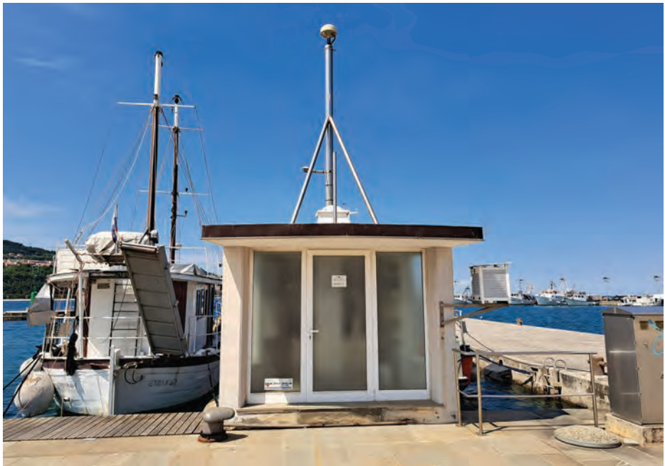
GNSS antenna of the SIGNAL network station on the roof of the Koper tide gauge station
