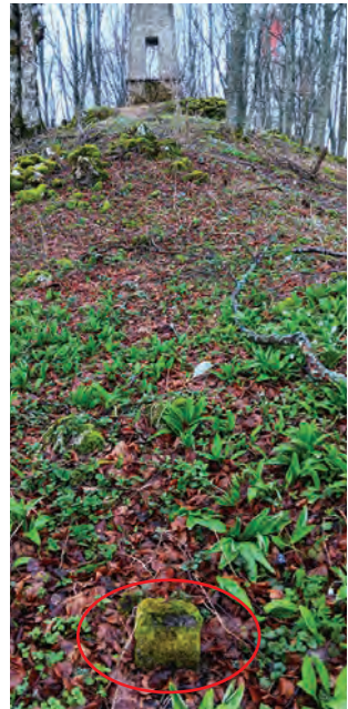
The lower reference point of the first-order trigonometric point Trdinov vrh today (left) and its appearance when it was erected in 1934 (right)
