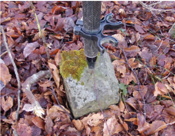
Medvednica (1024 m): forth-order trigonometric mark no. 532 in the trigonometric district of Postojna.
