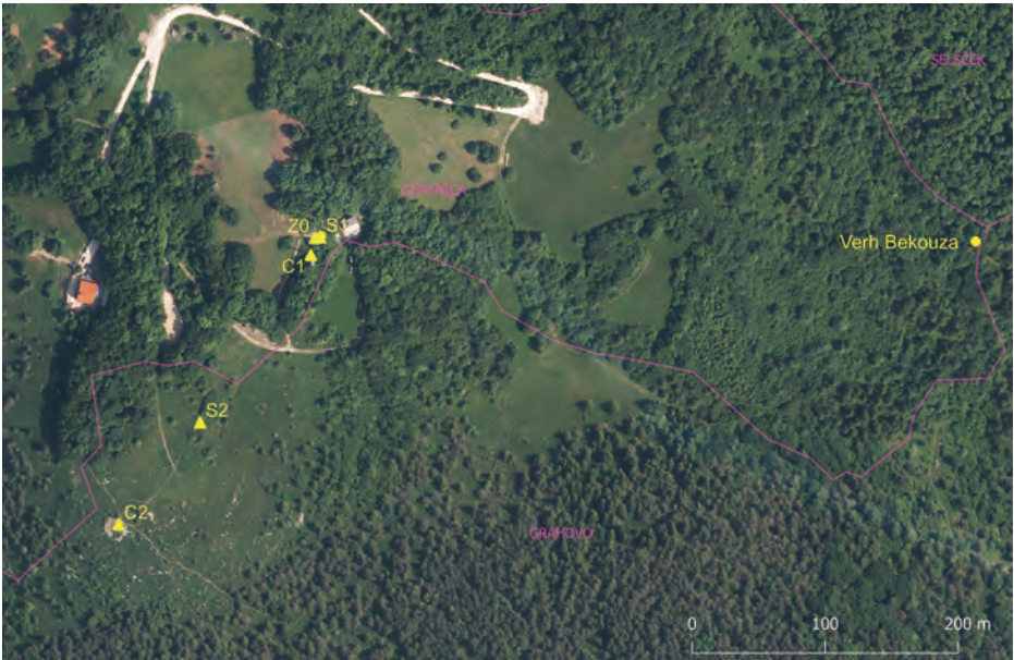
The physical marks of the second-order trigonometric point no. 301 on the national orthophoto.
