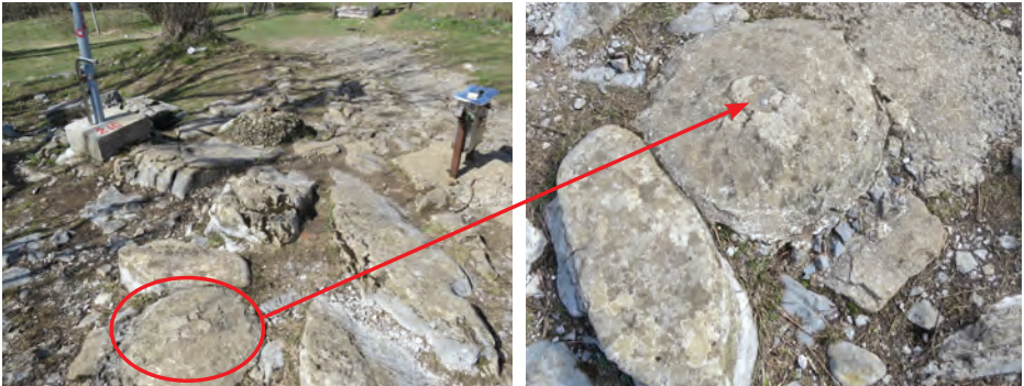
The main point Z0 of the second-order trigonometric point no. 301 is marked with a small metal pin.
