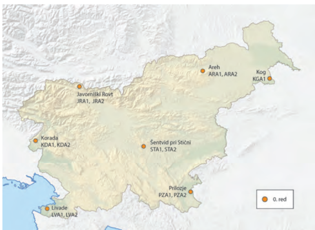
Locations of control points in the combined geodetic network and GNSS station designs.
