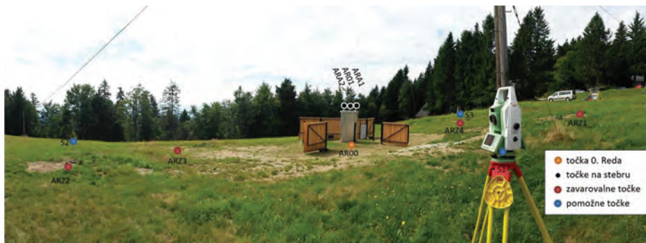
Carrying out geodetic control surveys at the AREH point.
