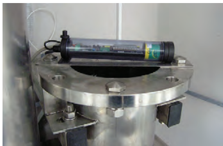
The reference point of the height coordinate system at the Koper tide gauge station (left) and instruments for measuring sea level – tide gauges (right).
